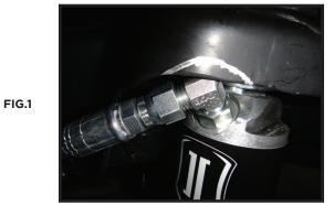
**7.** The hose must exit as pictured. [FIGURE 2] Allowing the reservoir hose to exit differently OR over tightening of the stem bushing lock nut will cause the reservoir fitting to collide into the frame. [FIGURE 3] Displays contact of the reservoir fitting and the frame when the shock is installed incorrectly.
